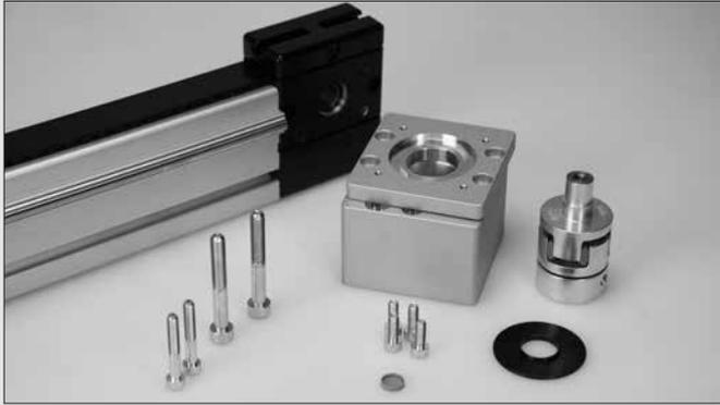
The torques transferred by the clamp connection factor in the maximum mating play for the shaft fits: Shaft k6 / hole H7. Force is transferred from the Coupling to the drive shaft by means of frictional resistance. The shaft and the hole in the hub must be degreased and cleaned to ensure a frictional connection for the drive.
