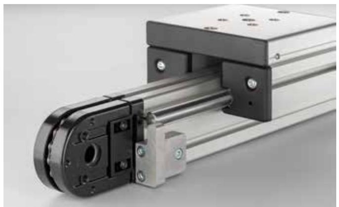
To fit Slide Stop LRE 8, first mark the desired end position on the support profile of the linear axis. This position does not need to match the maximum travel, but rather can be adapted to the transport task at hand.
