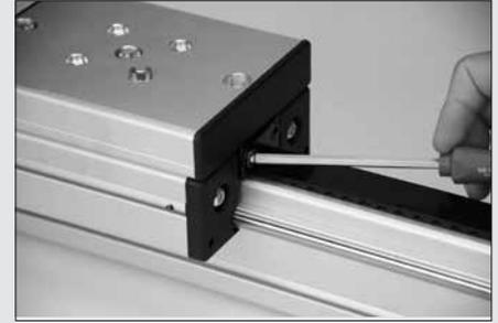
Insert both ends of the Timing Belt into the Tensioning Blocks so that the cavity inside each Tensioning Block is filled then screw securely into place. Fix one Tensioning Block in place under the carriage plate and use the other to tension the Timing Belt with the aid of the long Hexagon Socket Head
