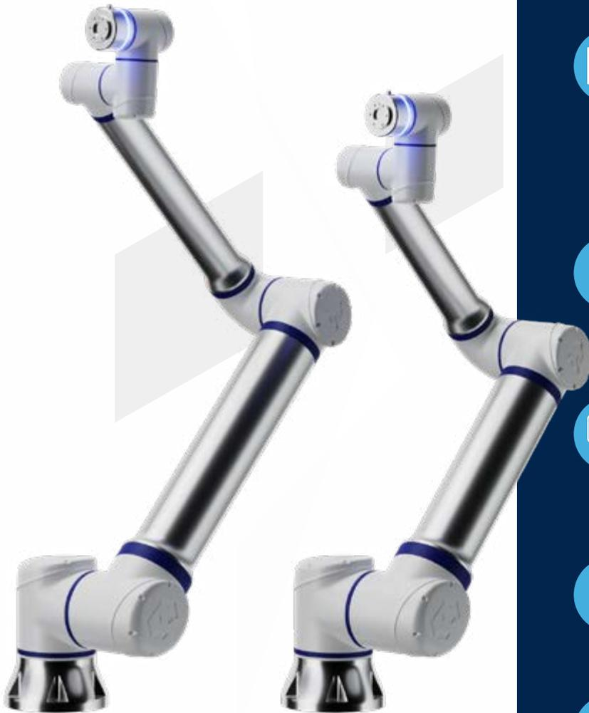
**CS620****CS625****20 kg****25 kg****1800 mm****1500 mm****±0,1 mm****±0,08 mm****3,9 m/s****3,3 m/s**
